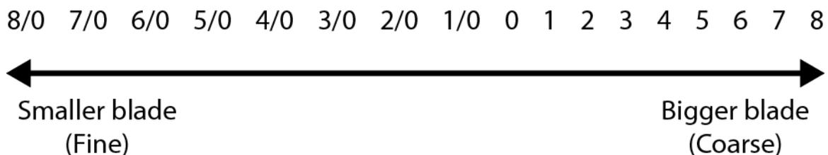
A size 8/0 is the smallest blade with the finest teeth and thinnest kerf<sup>1</sup>, while a size 8 is the largest blade with biggest teeth and widest kerf. It is important to select an appropriate sized blade for the work you are doing; you wouldn't want to cut a thick plate of metal with an 8/0 blade, nor would you want to cut a thin piece of 24g metal with a number 8 blade. Use the following chart to determine what size saw blade would be appropriate for the metal you intend to cut.
