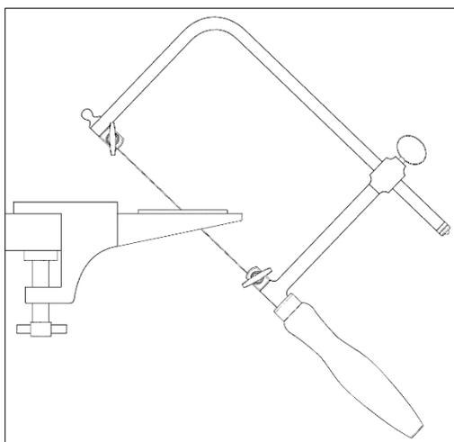
Holding the saw frame at a 90-degree angle to your work offers you the most amount of control when making complex curves and angles. However, if you want to cut a perfectly straight line then it helps to angle your saw frame forwards while cutting. (Pictured to the left.) This will increase how many teeth make contact with the metal at any given time, thus guiding the cut forward.
