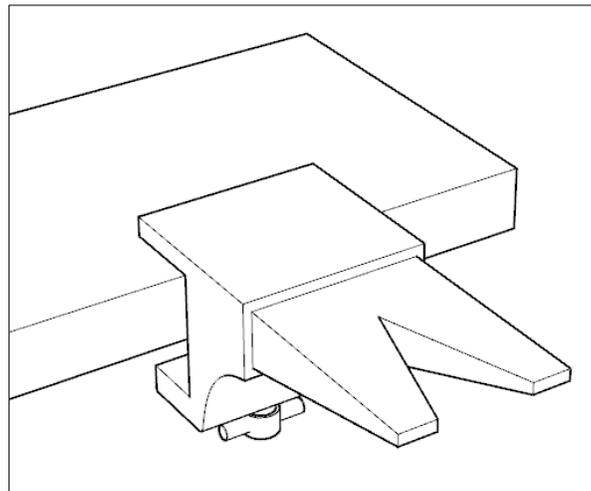
Place your metal on top of the V groove such that the metal is making contact with both sides of the V.
