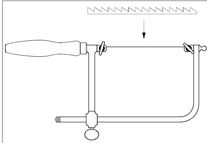
2. The saw blade should sit roughly in the middle of the upper jaw. (As pictured below.) If it isn't, release the tension knob, and adjust the spring arm by moving it up or down. Tighten the spring arm when this is achieved.
