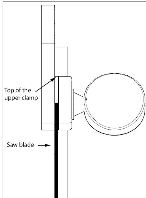
3. Compress the saw frame by pushing it against your bench, you should see the saw blade touch the top of the upper clamp. Tighten the knob on the upper clamp while the saw is still under tension to lock the blade in place.
