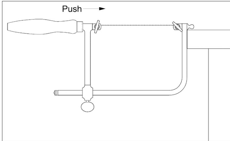
4. If done correctly, the saw blade will make a high “ping” sound when plucked. If it makes a dull sound instead, your blade is too loose. If this is the case, you may need more space between the top of the saw blade and the upper clamp. Adjust the spring arm accordingly and repeat the process. **It is critical that the saw blade is under an appropriate amount of tension to ensure that it cuts properly.**
